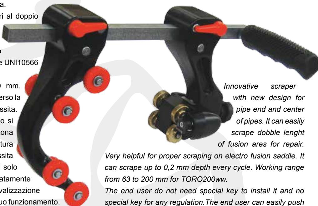
*Innovative scraper with new design for pipe end and center of pipes. It can easily scrape double length of fusion areas for repair.*
